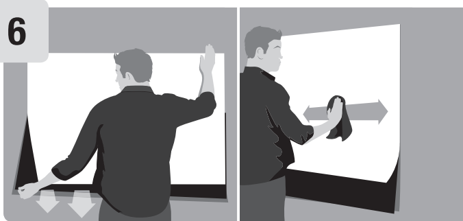
6 Continue to remove the liner 12" at a time and repeat step 5 until the surface is completely secured to the wall without air bubbles.
