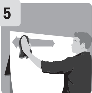
5 Using the cloth provided, start in the middle and push firmly against the surface moving any air bubbles to the edge.
